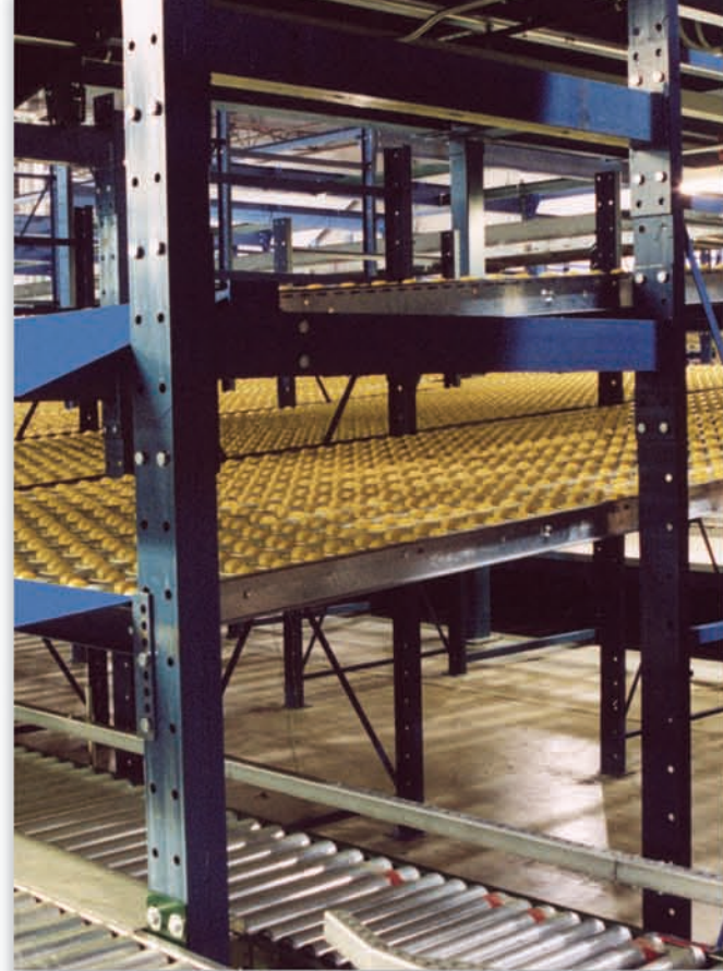
Connectors allow for 1" vertical adjustment
