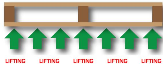
**Competitor's Twin Lift Bar Design Relies on Lifting Bottom Boards**
