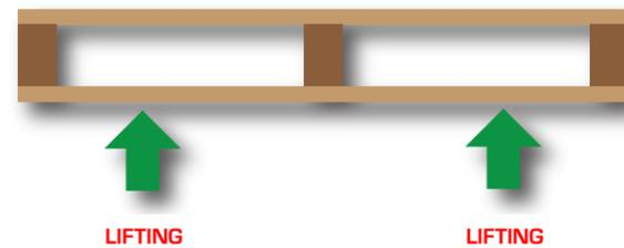
Four heavy duty ball bearings on each corner of the platform working with a screw-drive lift system respond to raise the deck lid up. The deck lid as a whole picks up the load, so that center stringers or blocks on pallets directly transfer the lifting force to the entire pallet. Lift performance is not dependent on bottom board strength.
