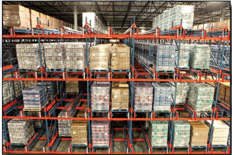
25-deep/40-wide Pallet Mole System utilizing 2-wide Cascade forklift attachment provides maximum density, 100% SKU selectivity & optimal productivity
