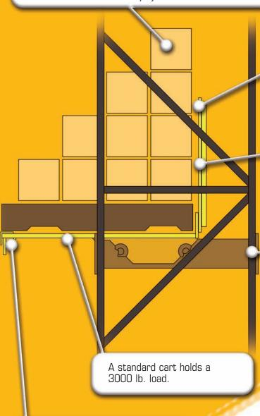
The order selector simply unlatches the cart and it rolls smoothly forward, allowing easy access to the product. The locking mechanism prevents the cart from rolling forward until it is approximately 50% empty.
